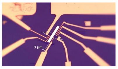
The image shows eight electrodes around a 20-nanometer-thick magnet (white rectangle) and graphene (white dotted line).
